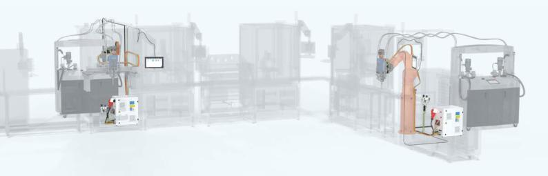
The new DispensingStation enables the dispensing system and dispensing monitoring system to be rapidly and reliably integrated as plug-and-produce elements. Portal axis systems (left) or robot applications (right) are used for integrating in existing production lines. However, the controller can also be used for manual dispensing processes.
